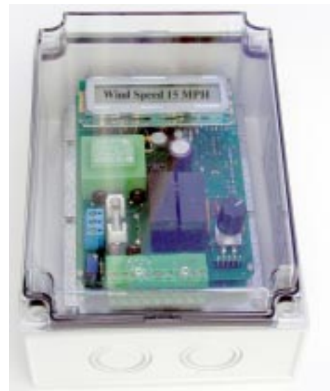
Zephyr in Weatherproof Enclosure
