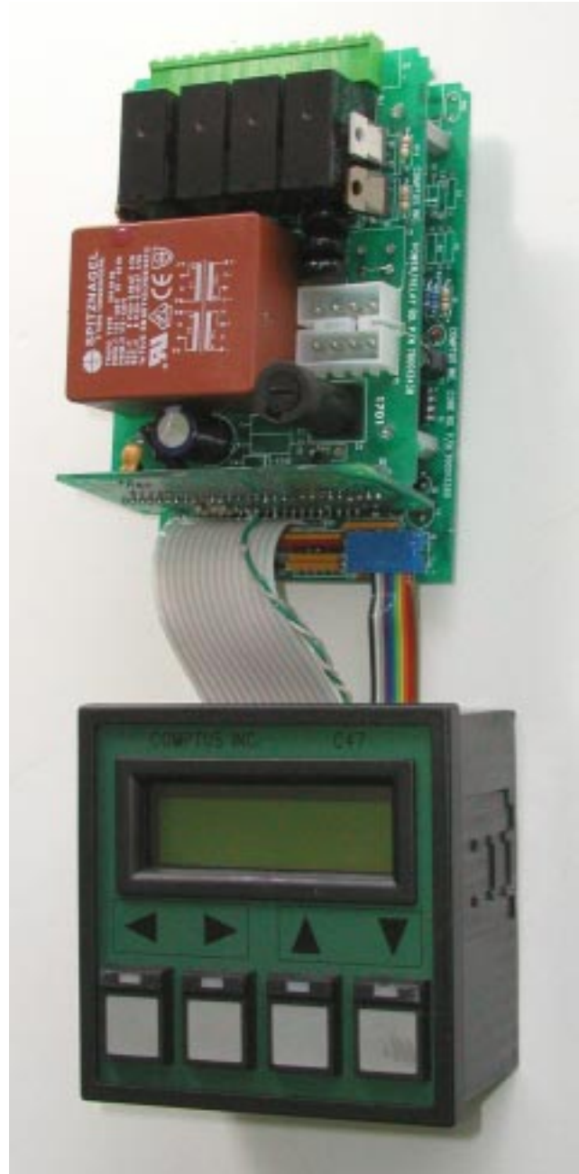
C47 Sub-Panel Mounting 3.75 inch Square Panel Cut Out 3 Inch Mounting Depth Recommended for portable installations subject to mechanical shock
